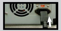
The plug end should be plugged into a surge protector which is then plugged into an electrical outlet.
