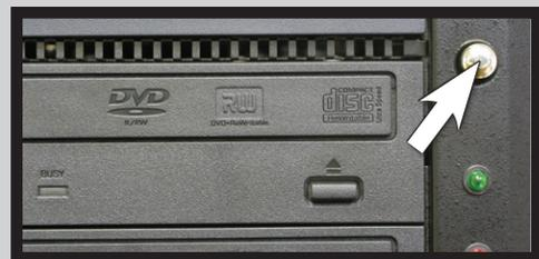
4. Allow the system to boot up. When ready, **1. Copy** should appear on the LCD screen.
