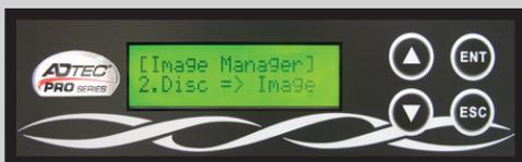
Press **ENT**. After several seconds, the screen will show the image from your master is loading and the progress of the load.
