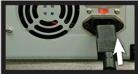
The plug end should be plugged into a surge protector (not included) which is then plugged into an electrical outlet.
