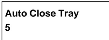
Here 5 means that it takes 5 seconds to close the writer's tray automatically after copying finishes and the tray is ejected. Besides 5 seconds, there are 10, 15, 20, 25, 30, 35, 40, 45, and 50 seconds for choice. If you have set one or all seven writers in function 11.5, and choose 10 seconds here, then one writer's tray or all seven writers' trays will be closed in 10 seconds after copying finishes.
